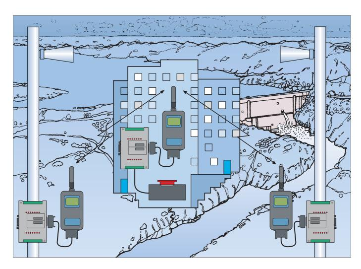
At hydropower stations, water level of the reservoir is subject to strict monitoring and control. Excess water is at times released through the bypass channel, for various reasons. In order to avoid accidents, it is customary to warn the public by sounding sirens before the release.
