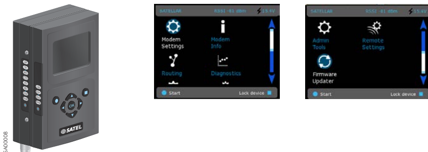
Figure 5.4 RU together with Central Unit (CU) equipped with LCD display and keypad, the main views
