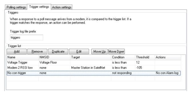
Figure 35: Trigger settings view
