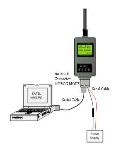
Figure 2: Full operation connections
