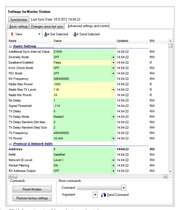
Figure 25: Modem settings view: Advanced settings and control
