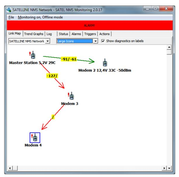
Figure 39: NMS PC Monitoring, Main window
