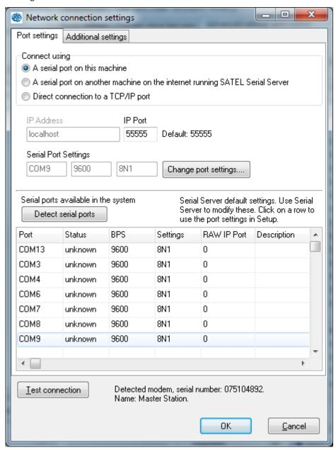
Figure 26: The Connection settings window showing Port settings tab
