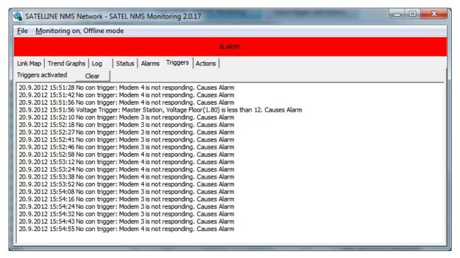
Figure 46: Triggers tab
