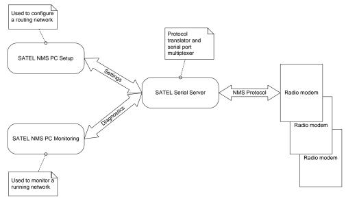
Figure 1: Components of the SATEL NMS solution
