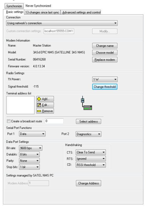
Figure 23: Modem settings view: Basic settings
