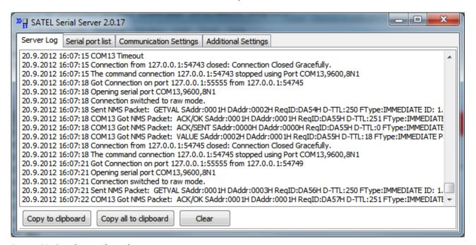
Figure 48: Serial server log tab
