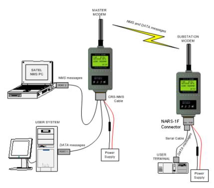
Figure 4: Serial connections in a deployed NMS network
