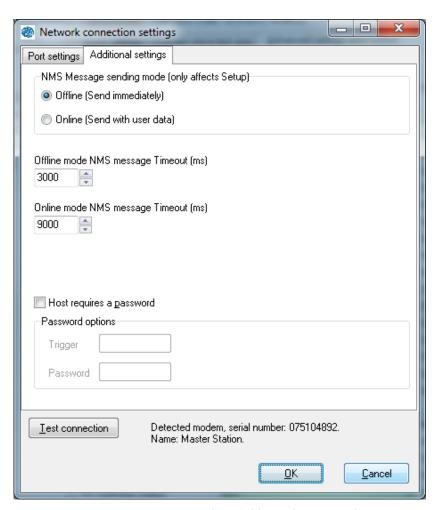
Figure 27: Connection settings window: Additional settings tab
